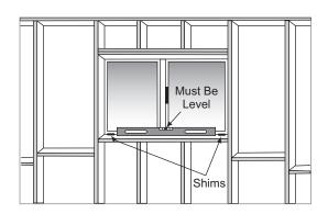
NOTE: DO NOT Shim directly under the vinyl window frame. Shim between the sill plates.
